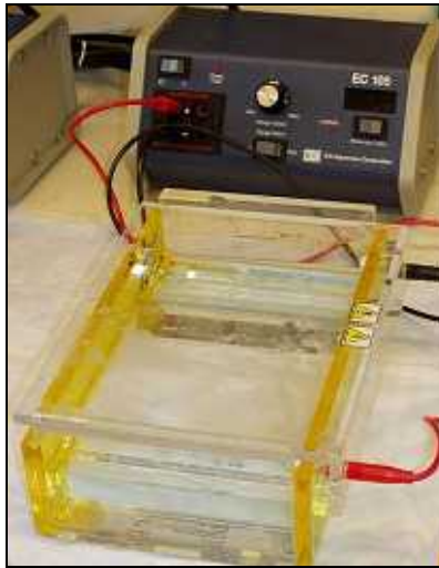
Figure 6. Gel electrophoresis unit (or gel rig): power supply and buffer tray containing an agarose gel. (Accessed at 10:45 hrs, 2/4/09 by internet at http://en.wikipedia.org/wiki/Gel_electrophoresis )
