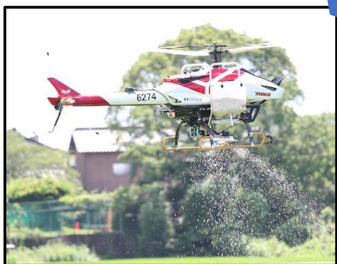
Map-based variable rate fertilization according to growth
