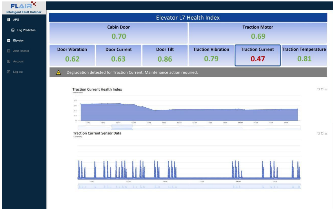
FLAIR's Intelligent Fault Catcher utilises IoT sensors to monitor the operating condition of industrial equipment and predict upcoming faults.
