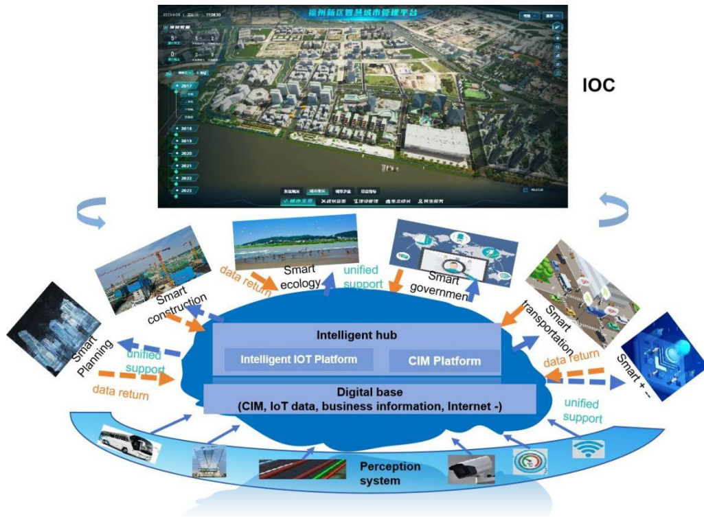
The IOC and Smart application systems are built based on the same foundation, such as intelligent hub and digital base
