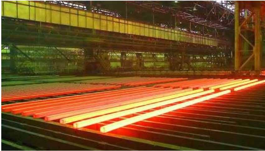
Figure 30 Harsh Environment Makes it Difficult to Install Sensors or Communication Device
