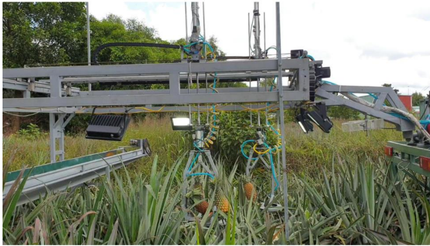
Figure 54 The Pineapples Harvesting Robot working in the Field
