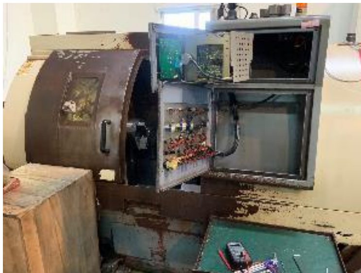
Figure 29 Legacy Machines That Lack of Communication Interface
