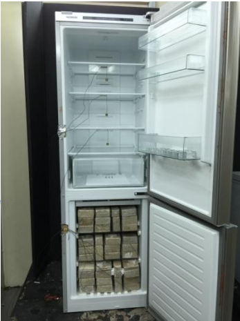
Test loading view of frost free refrigerator-freezer
