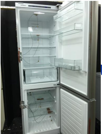
Test loading view of frost free refrigerator-freezer
